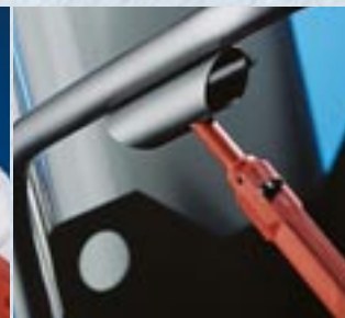
Integrated torch holder on the trolley
